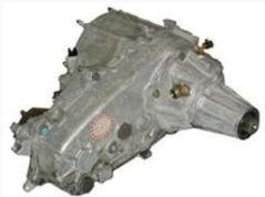
The NP 207 is one of the weaker Jeep transfer cases, but can be upgraded. The NP 207 has an aluminum case and chain driven planetary reduction. Thankfully the NP 207 was installed behind some of the weakest Jeep power trains every used. It featured a 2.60:1 low range and a straight through design high range, but featured a driver side front output. It was used in one year of the Jeep YJ Wrangler 1987, and in the early XJ Cherokee's from 1984-1987.
