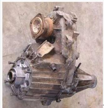
The NP 208 is similar to the NP 207 as it has an aluminum case and chain driven planetary reduction. It uses a 23-spline input shaft and has a driver's side front output. The NP 208 has a low range of 2.62:1 and features a straight through rear output. It can be identified by a silver tag on the rear that reads "New Process Gear Model 208". It was used in full sized Cherokees from 1980-1983 and in Jeep trucks from 1980 to 1987. The NP 208 was the Command Trac option for the Jeeps of this period.
