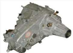
The NP 219 was an option in 1980-1982 full size Jeeps. It functions much like the early Quadra-Trac and has been nicknamed the "fake" Quadra-Trac as New Process Gear and not Borg Warner built it. It uses a viscous clutch assembly and vacuum actuation. Not many of these are still in use, rebuilt parts are getting hard to find, and the overall strength is not that great.
